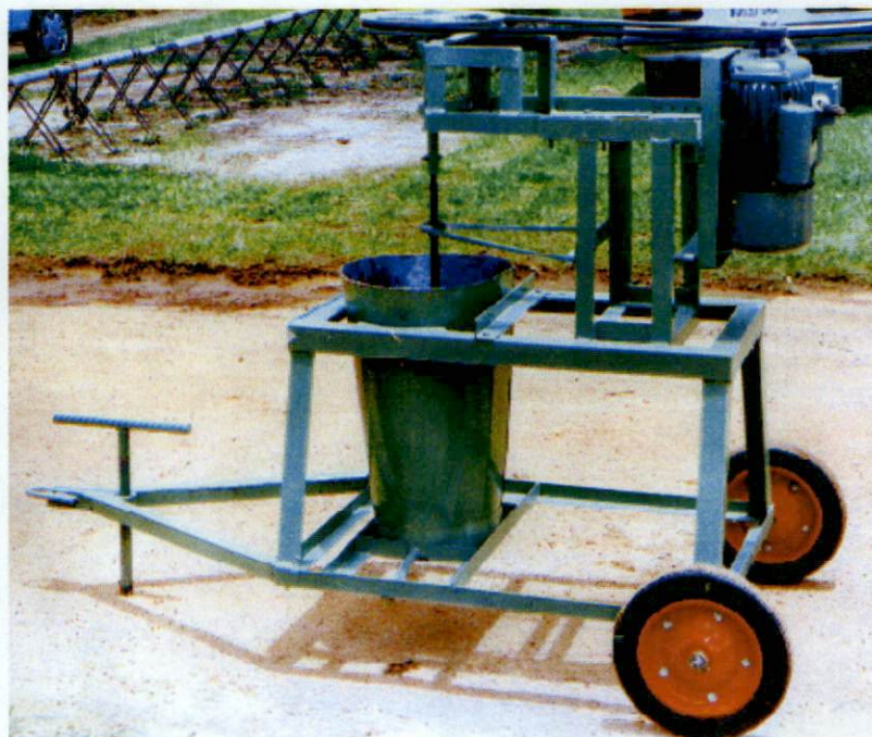
Traditional and Mechanized groundnut oil extractors developed by the Institute of Agricultural Research, Ahmadu Bello University
