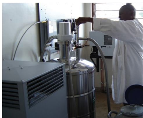
Liquid Nitrogen Plant that produces Liquid Nitrogen which keeps the vaccine in the required cool temperature for preservation
