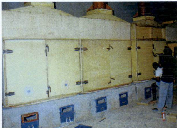
Figure 3: multipurpose gas dryer used by community based organizations for processing mango and other agricultural products
